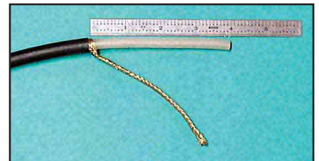
Figure 5—Preparation of the coax trap ends.
