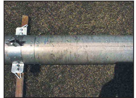
Figure 4—The guy clamp attached to the main element.
