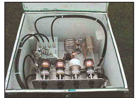
Figure 14—L-network for 160 meters (right of center) and 80 meters (far right of center).
