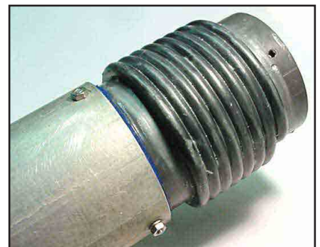
Figure 7—The 80 meter trap installed on the main element.
