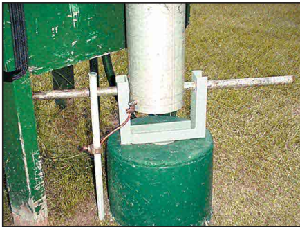
Figure 12—Two views of the pivot fixture for positioning the base insulator.
