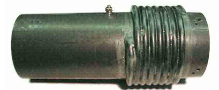
Figure 6—Completed 80 meter trap assembly ready to install.
